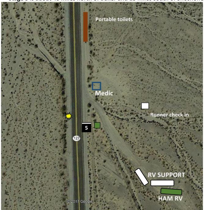
For 2022 a light tower will be delivered and set up. It appears that the best location to set up is directly across Highway 127 from the exchange point. The lights need to be adjusted before raising the tower so that they aim directly across toward the exchange point and the lights do not interfere with cars coming in either direction.
